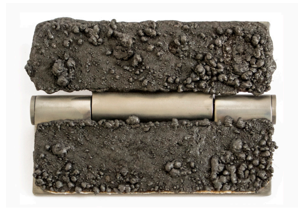
Butt hinge following activation of the intumescent pad
